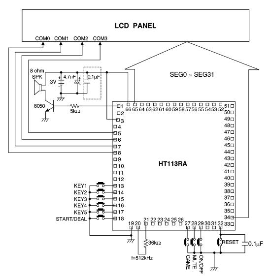
Note: The capacitor in the dotted block is recommended. The IC substrate should be connected to VSS in the PCB layout artwork.
